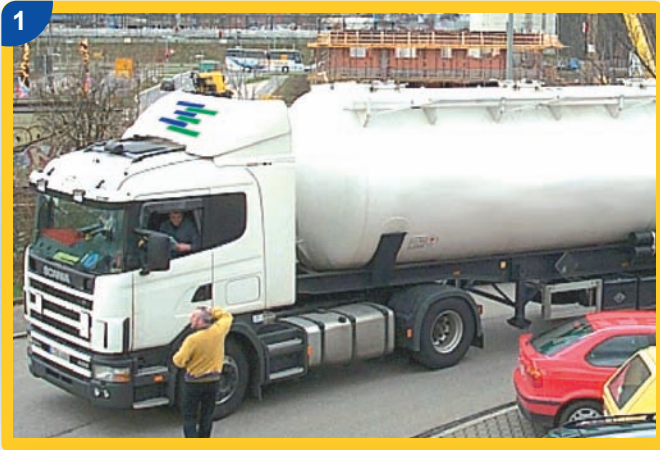
1 Silo pressurised vehicles
