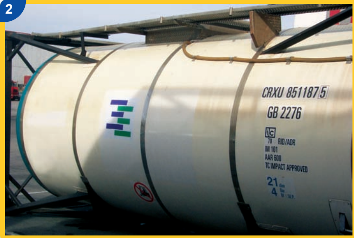
20 foot intermediate bulk container prior to the shipment of chemical fluids in Tarragona.
