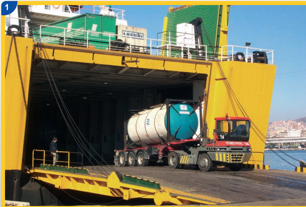
Intermediate bulk container with (MDI) in the harbour of Barcelona for shipment to Genoa (Italy).
