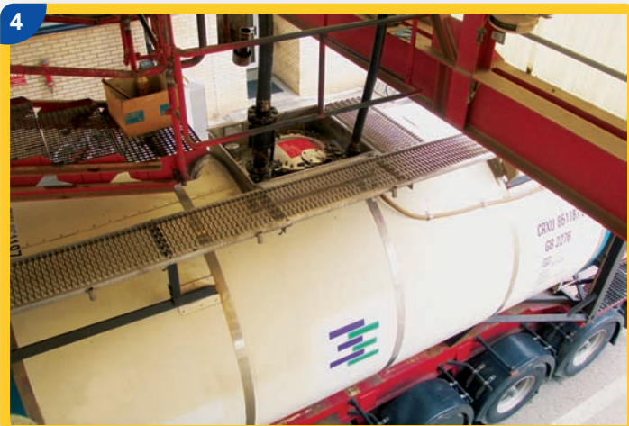
Bulk container following completion of the loading process in the chemical plant.
